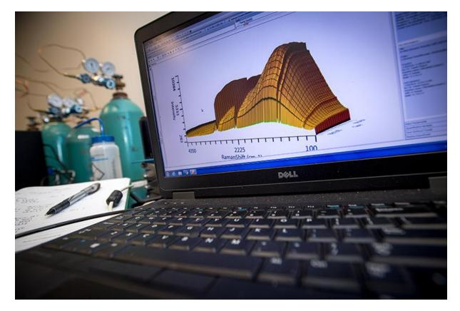
Using a Raman spectroscopy, a laptop in the lab of Daniel Shantz in the Department of Chemical Engineering displays a spectrum of reacted benzene. This technology allows scientists to better understand the mechanism of chemical reactions.
