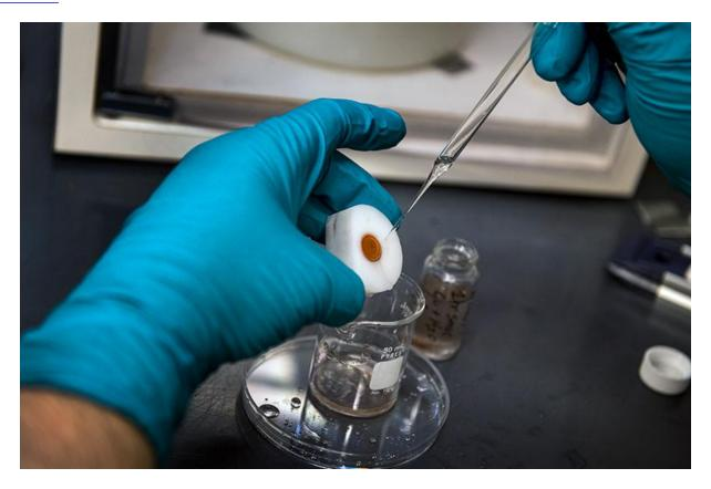
After creating eroded copper particles, Jeremy Wright, a doctoral candidate working in the lab of professor Brian Mitchell in the Tulane Department of Chemical and Biomolecular Engineering, transfers the particles for analysis to determine if nanoparticles are present. The nanoparticles will eventually be used to create metal-based 3D printed objects with finer features.
