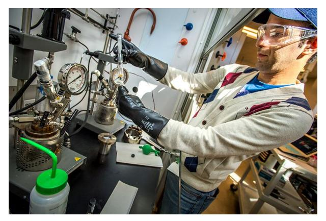
Meysam Shahami, a doctoral student in the Department of Chemical Engineering, extracts reacted benzene in the lab of Daniel Shantz. The solution will be used to analyze how much phenol is produced using a one-step reaction. Researchers hope to simplify the process of producing phenol which is used to make soft and hard plastics.
