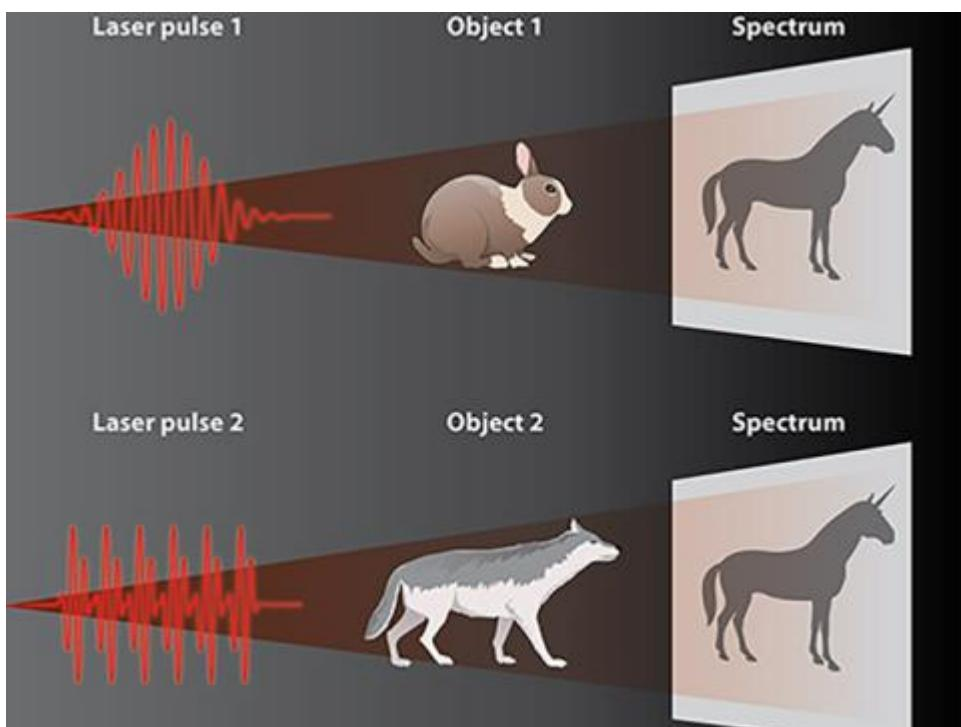
This image illustrates a newly proposed mimicry scheme relating to or derived from the electromagnetic spectrum of visible light by which researchers could make two different materials mimic each other's spectra — or produce the spectrum of other, more exotic materials. (Image courtesy APS/Carin Cain)
